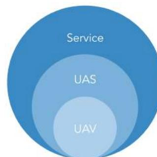
Most of the UAS are controlled within VLOS (visual line of sight). Some can fly BVLOS (beyond visual line of sight) and/or completely autonomous. In autonomous flight mode, a UAV follows a predetermined flight plan and relies on its sensors to fulfill the mission. The flight is usually controlled or observed via telemetry.
